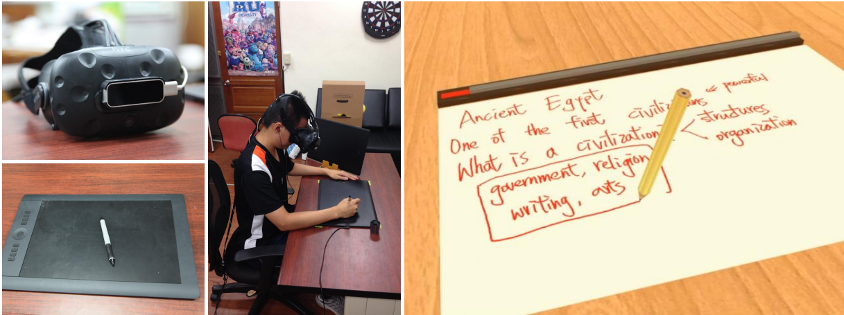
Figure 1: We present iVRNote, an interactive note taking interface, to help students study video lectures in VR (middle and right). To enable students to take notes in VR (right), we install a digital tablet (bottom left) on the desk and track a stylus's position and orientation using the tablet's interface and the leap motion controller (top left).
