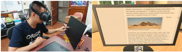
Figure 5: Students can check the Wikipedia page on a display on their desks in the virtual classroom, if they encounter difficult words and terms in a lecture. (Left) The student scrolls the web page by swiping his finger on the virtual display that is physically co-located with a Wacom tablet for passive haptic feedback. (Right) The Wikipedia web page is shown in the VR classroom on a virtual desktop computer.
