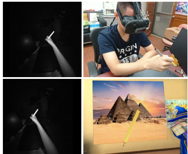
Figure 2: (Left) Stereo infrared images captured by the leap motion controller. (Top right) The photograph shows how the user holds the physical stylus. (Bottom right) We track the stylus' position and orientation in the physical environment and shows the virtual stylus in the VR classroom.
