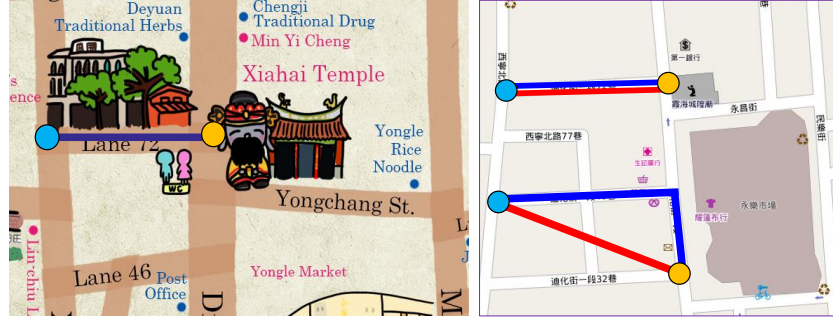
Fig. 3. The Euclidean (red lines) and road (blue lines) distances between nodes are considered to measure matching quality. In this example, we show two possible matchings of the blue and the orange nodes on the two maps. The bottom matching is apparently incorrect because of distance inconsistency.
