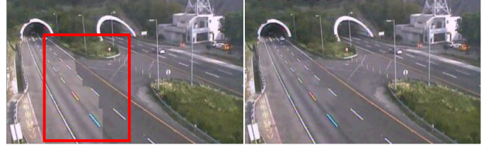
Figure 7: Left and right show the comparison without and with Poisson blending. (Left) Discontinuity artifacts occur when videos with different illuminations are composed, as highlighted by the red rectangle. (Right) The artifacts are removed by our smoothing.
