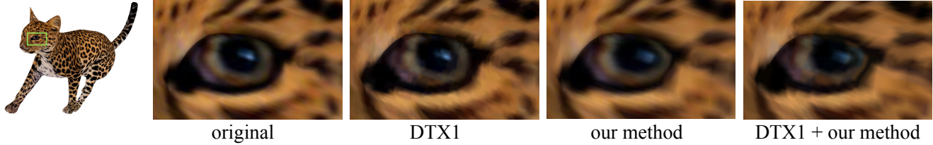
Figure 11. We render the model with the original texture and the textures compressed by DXT1, our method and DXT1 + our method. In this example, the texture is compressed to have 16.67% and 50% of the original size using DXT1 and our method, respectively. Note that the compression ratio of DXT1 is uncontrollable so that some features are distorted after the compression. We also show that a texture can be compressed by DXT1 and our method simultaneously to achieve a better compression ratio (8.33% of the original size).
