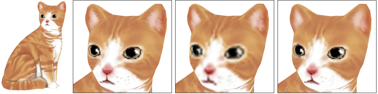
Figure 8. From left to right are the cat model, the cat's head rendered with the original, down sampled, and our compressed textures. Both the compressed textures have 57% of the original size. Compared to the down sampled texture, our result suffers from less aliasing artifacts when the camera is very close to the cat's face.
