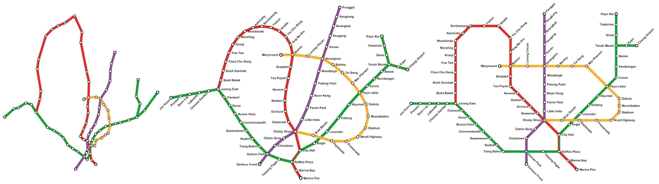
Fig. 1. From left to right are the geographic, curvilinear and octilinear metro maps of Singapore. We provide users with an intuitive interface to edit the map. The criteria for a visually pleasing result, such as evenly spaced stations, smooth/straight transportation routes, and maximal included angles at junctions, are satisfied.
