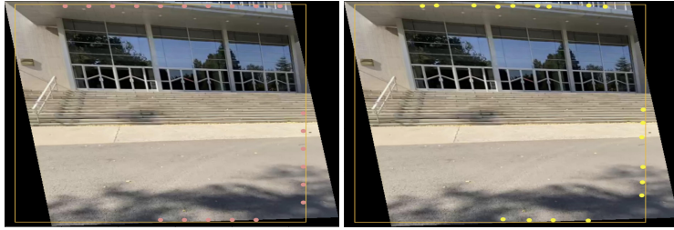
Fig. 3. In this example, source and target images are represented using a bitmap form and a rectangle. (Left) Control points are uniformly sampled at the boundary of the overlapping area. (Right) Points are adjusted to high gradient positions for better alignment around structural regions. Note that control points are used to warp the outer region of a source image, and the points in the bottom left corner are unnecessary.
