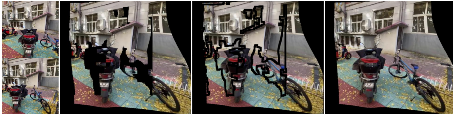
Fig. 2. We fill in the holes after warping the source image using optical flows. The left side shows the source and target images. In the middle left, the source image contains holes. In the middle right, we start by filling the middle part of the hole by directly copying pixels from the target image, since the two images are in the same coordinate system. Finally, on the right, we use an inpainting technique to fill the gaps around the hole’s boundary to minimize potential visual artifacts, as no optical flow estimators are perfect.
