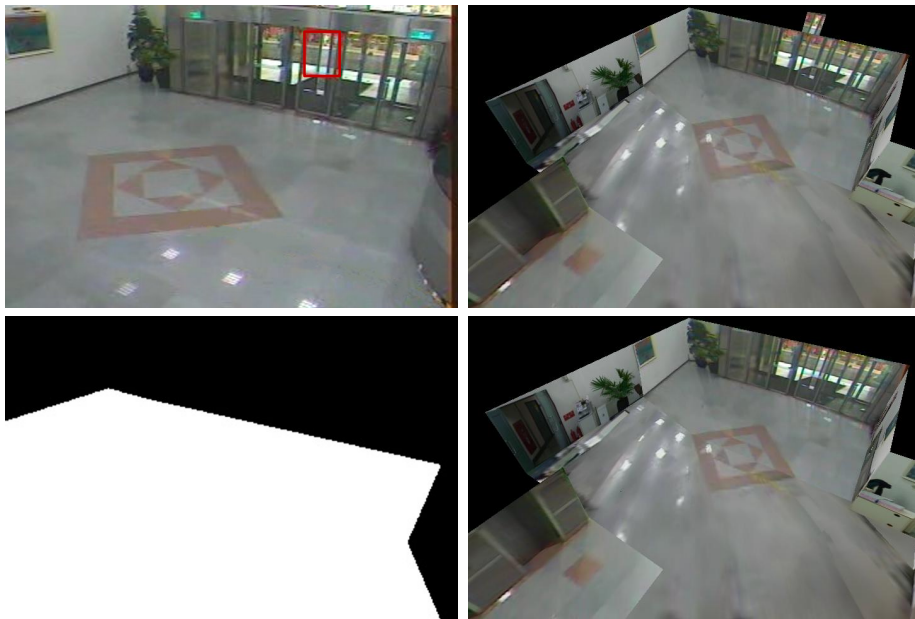
Figure 12: Dynamic background removal by ground mask. There is an automated door in the scene (top-left) and it is visualized by a billboard (top-right). A mask covered the floor (bottom-left) is used to decide whether to visualize the foreground or not. With the mask, we can remove unnecessary billboards (bottom-right).
