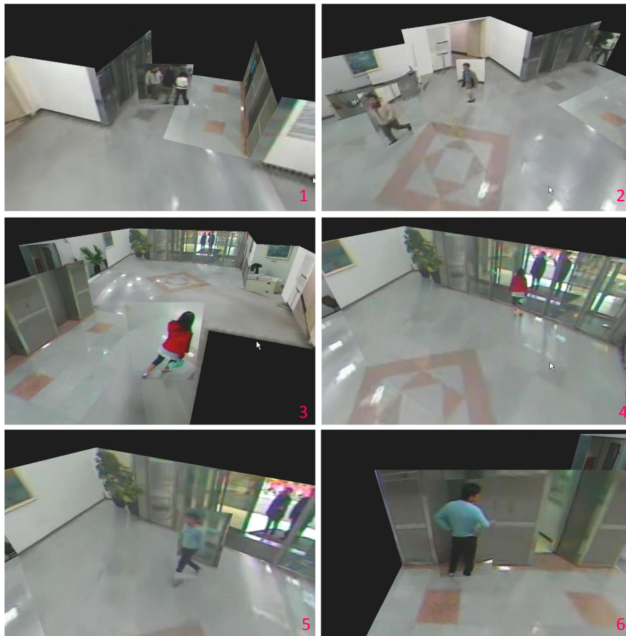
Figure 13: Immersive monitoring at arbitrary viewpoint. We can zoom out the viewpoint to monitor the whole surveillance area or zoom in the viewpoint to focus on a particular place.
