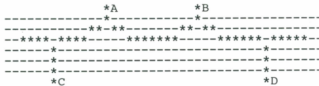
Figure 4. Noise points A, B, C, and D cause heavily shape variations. Symbol '*' denotes the obtained skeleton, while symbol '-' denotes the removed points.
