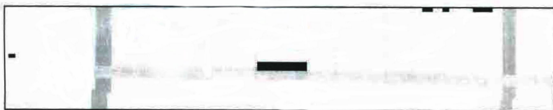
Fig. 7. The gray pixels belong to form frames, and black pixels which are attached to the horizontal frame are noise that also need be removed.
