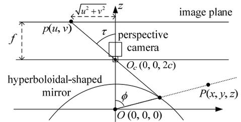
Fig. 3. Catadioptric omni-camera structure and its camera coordinate system.
