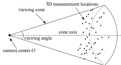
Fig. 14. An illustration of finding the optical axis and the viewing angle.
