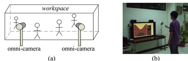
Fig. 1. Stereo vision system with two omni-cameras for this study. (a) Illustration of the vision system. (b) A user playing a game using the system.
