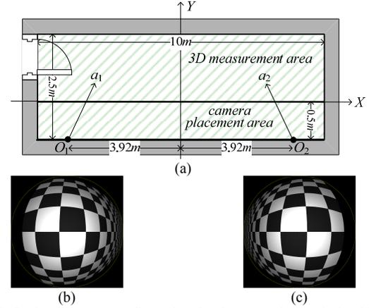
Fig. 15. Optimal system configuration for the general case derived by the optimization process proposed in Section VI. (a) An illustration of the optimal system configuration. (b)(c) Simulated images taken by the two cameras, with 3D measurement area drawn as a checkerboard cube.
