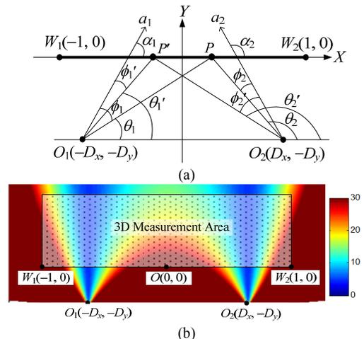
Fig. 8. Analysis of function  $E_w$ . (a) Illustrations of related terms. (b) Drawing of distribution of measurement errors  $E$  of a configuration.
