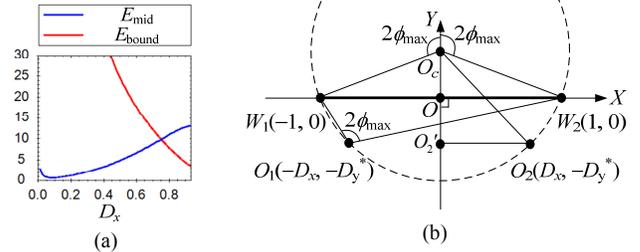
Fig. 10. Illustrations of finding the optimal solution  $D_x^*$  and its upper bound. (a) Plot of  $E_{\text{mid}}$  and  $E_{\text{bound}}$  versus  $D_x$  when  $D_y^* = 0.1$  and  $2\tau_{\max} = 60.0^\circ$ . (b) Derivation of the upper bound of  $D_x$ .
