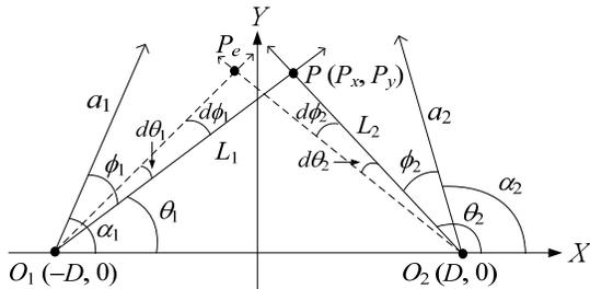
Fig. 6. Top-view illustration of triangulation process and error propagation.
