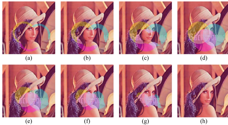
Fig. 5. Illustration of pixel processing order in watermark embedding and removal. (a)–(d) Intermediate results of image watermarking when 25%, 50%, 75%, and 100% of the watermark pixels have been processed, respectively. (e)–(h) Intermediate results of image recovery when 25%, 50%, 75%, and 100% of the watermark pixels have been recovered, respectively.
