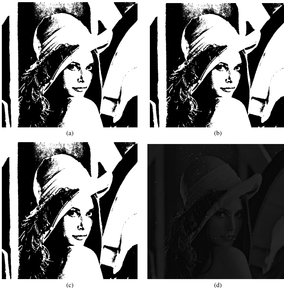
Fig. 6 Input binary images, output stego-images with message data, and the difference images. (a) Binary image “Lena”. (b) The stego-image using the greedy search algorithm and the optimal encoding table. (c) The stego-image using the DPA and the optimal encoding table. (d) The difference image between (a) and (c) in which the white spots are difference pixels.
