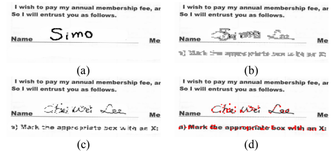
Fig. 12. Authentication result of document image of a signed paper attacked by painting white color on the original signature and texts, and replacing the signature by a fake one in Fig. 6(b). (a) Tampered image yielded by the painting operation. (b) Result with tampered blocks detected and marked as gray. (c) Data repair result (d) Data repair result with red dots indicating unrepaired blocks.
