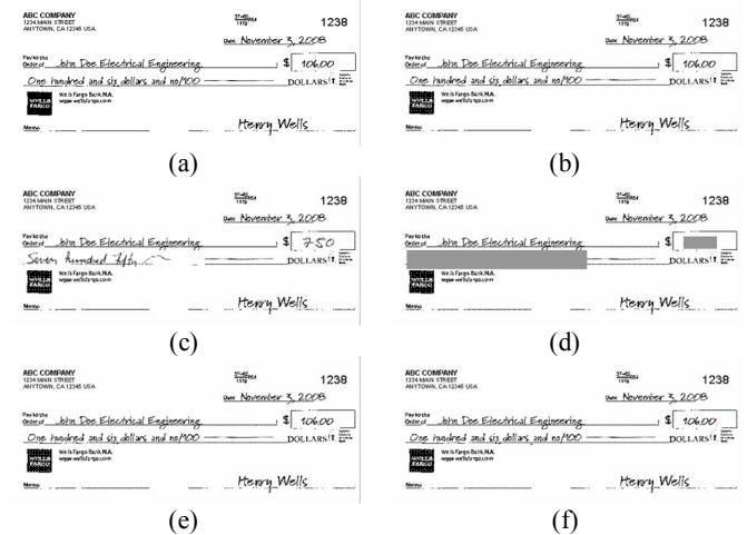
Fig. 15. Authentication result of an image of a check in PNG format attacked by superimposing counterfeit number “750” located at right side and text “Seven hundred fifty” located at left side. (a) Original cover image. (b) A stego-image with embedded data. (c) Tampered image by the superimposing operation. (d) Result with tampered blocks detected and marked as gray. (e) Data repair result. (f) Unrepaired pixels shown in red (none for this example).
