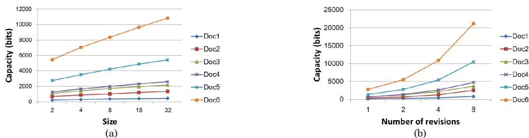
Fig. 10. The embedding capacities. (a) Embedding capacities of documents with chosen sets of different sizes. (b) Embedding capacities of documents with different number of revisions.
