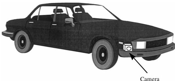
Fig. 1. Illustration of a vehicle mounted with a camera for imaging lateral views.
