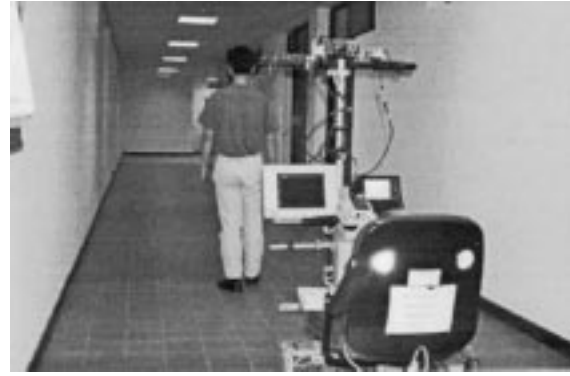
Fig. 9. The vehicle is guided automatically to follow a person who walks in front of the vehicle.
