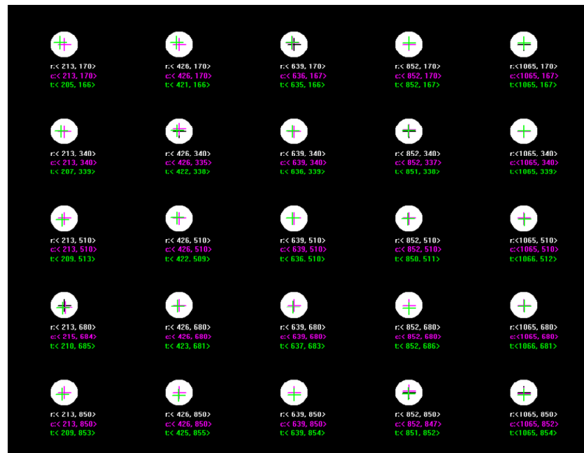
Fig. 14. Comparison using re-captured image points. The precise landmark position, the computed position by proposed method, and that by Tsai's method are listed under each dot.
