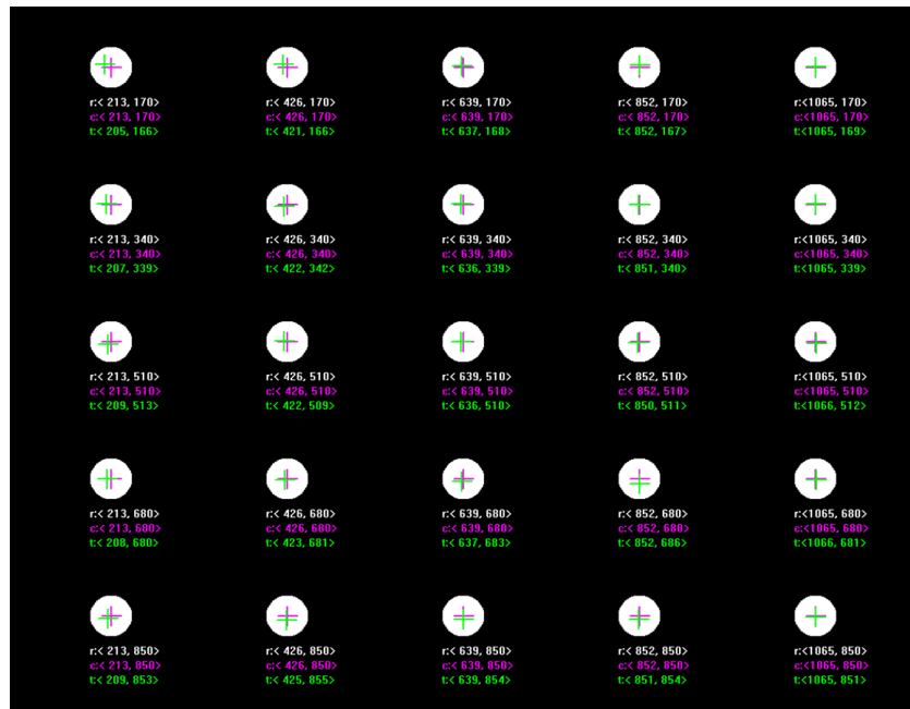
Fig. 13. Comparison using calibration image points. The precise landmark position, the computed position by proposed method, and that by Tsai's method are listed under each dot.
