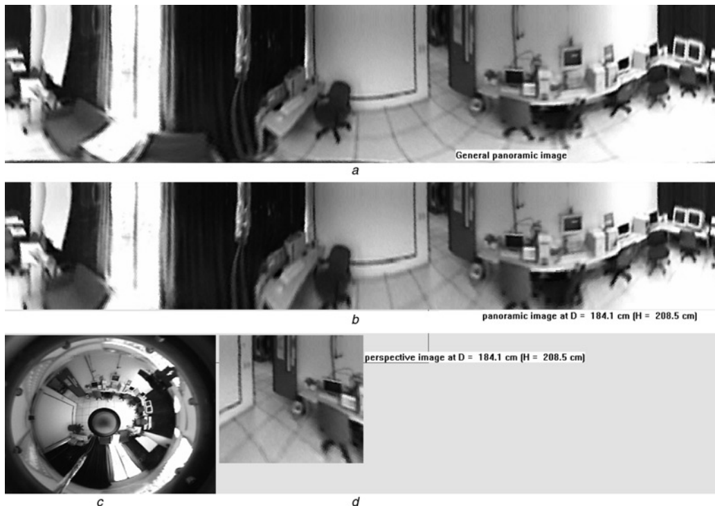
Fig. 8 Examples of image unwarping a Generated generic panoramic image b Generated panoramic image at distance 184.1 cm c Original omni-image d Generated perspective-view image
