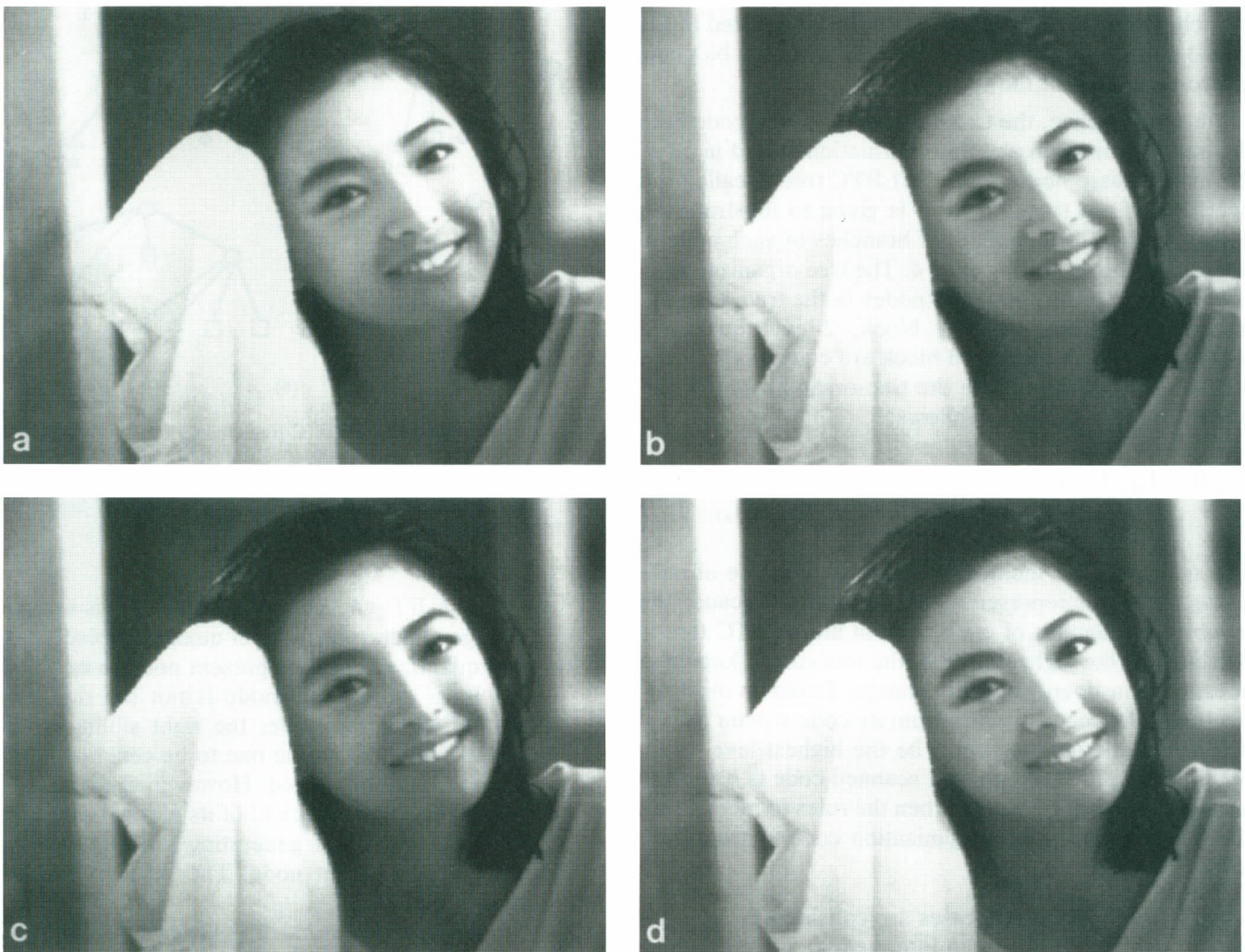
FIG. 7. Example of reconstructed images for three different methods (I). (a) Original image GIRL with 8 bits/pixel; (b) image reconstructed image by BTC with MSE 8.70 and 1.6 bits/pixel; (c) image reconstructed by AMBTC with MSE 8.07 and 1.6 bits/pixel; (d) image reconstructed by AMLBTC with MSE 3.07 and 1.6 bits/pixel. The MSE value of the proposed AMLBTC is much lower than those of the other two methods under the same compression ratio.
