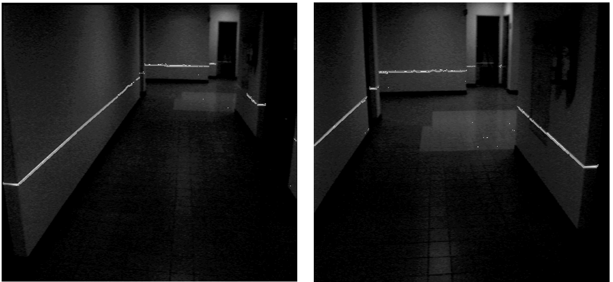
Fig. 9. Two examples of image processing results. The pixels in candidate set are shown as white spots, and the extracted environment features are shown as gray line segments.
