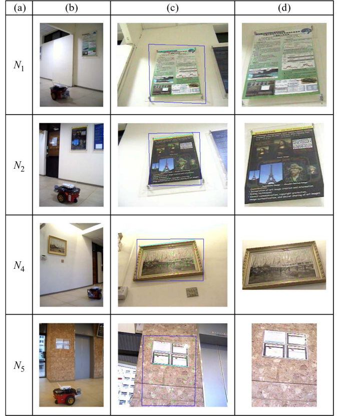
Fig. 8. Experimental results of object monitoring and path correction at four selected path nodes. (a) Labels of monitored objects. (b) Vehicle monitoring the objects at the nodes. (c) Matching results and the calibration lines used for path correction. (d) Images of the learned objects.
