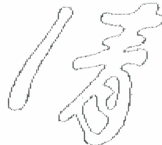
(c) Output image resulting from detection identical to that of (b) except that the curved edge detection is additionally applied to some of 24 neighboring points of origin of each detection circle in (b) in which curved edge pattern is not detected.
