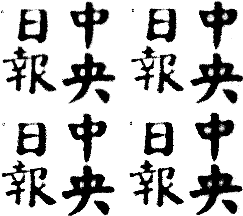
FIG. 14. Noniterative sharpening results of a character image: (a) the blurred image; (b) sharpening result for n = 3 ; (c) sharpening result for n = 5 ; (d) sharpening result for n = 7 .
