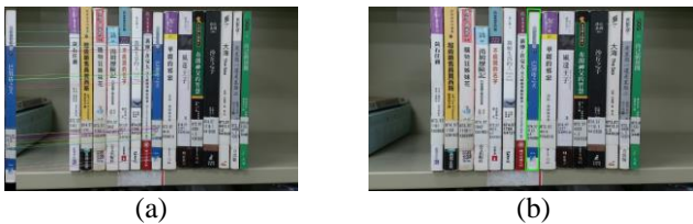
Fig. 5: Results of book spine recognition. (a) Result of matching a book-spine image (appearing as left slim part in figure) with an input image. (b) The green bounding box encloses the correct book spine.
