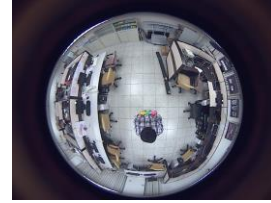
Fig. 6: A clear multicolor edge mark (the yellow-green-pink strip) in the acquired omni-image.
