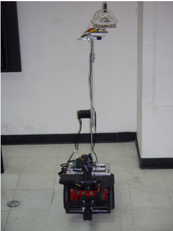
Figure 7: All the experimental images were taken by an autonomous land vehicle quipped with an upward-looking omni-directional camera.
