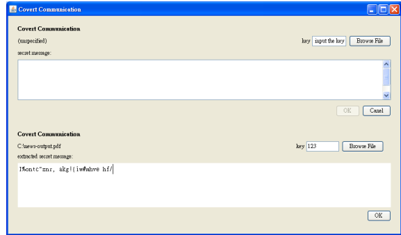
Figure 9 Window of user interface with a wrong key as input, resulting in erroneous extraction of embedded message.
