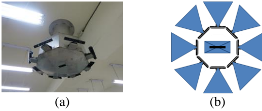
Fig. 1 The octagonal 9-KINECT imaging device designed for use in this study. (a) The exterior appearance. (b) The placement of the 9 KINECT devices.
