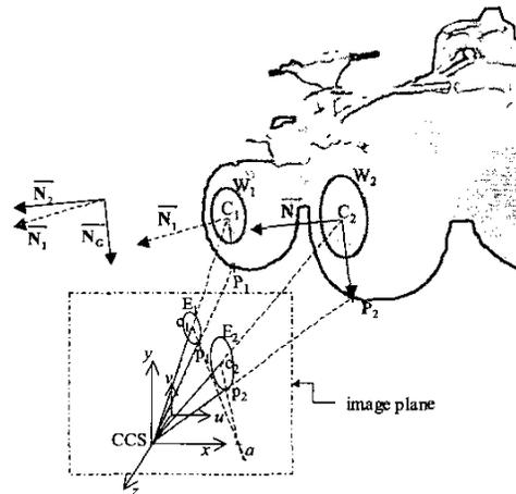
Figure 3. The projection of two wheels and the notations used in this study.
