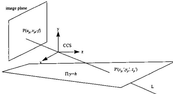
Figure 5. Illustration of the back-projection principle for finding the space point corresponding to an image pixel.
