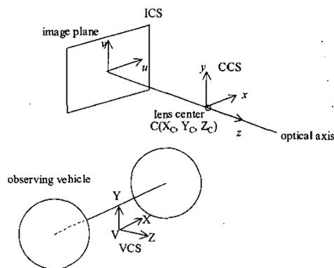
Figure 4. The coordinate systems used in this study, including the camera coordinate system  $x-y-z$ , the image coordinate system  $u-v$ , and the vehicle coordinate system  $X-Y-Z$ .
