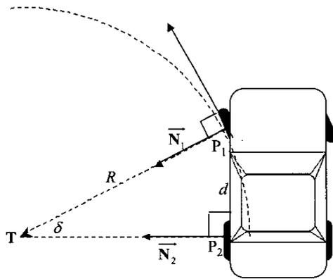
Figure 6. Vehicle Kinematics.
