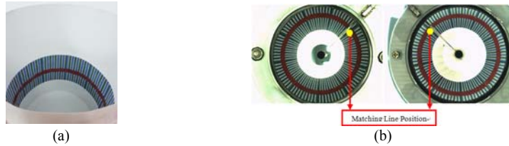
Fig. 8. Illustration of finding corresponding matching lines manually by visual inspection. (a) Grid pattern wrapped into a cylinder. (b) Corresponding matching lines in two omni-images.
