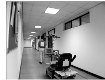
Fig. 11. The vehicle is guided automatically to follow a person who walks in front of the vehicle.
