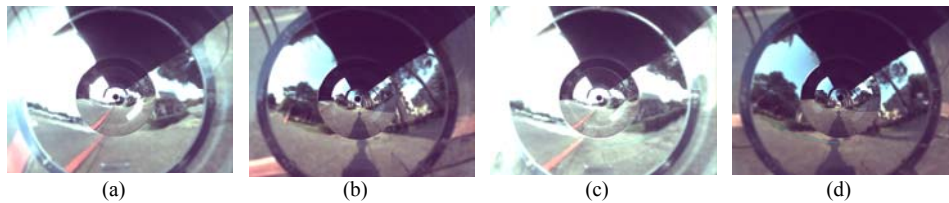
Fig. 13. Results of lawn corner detection and localization. (a) and (b) Lawn images taken in two perpendicular directions. (c) and (d) Lawn boundary detection results.
