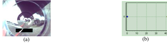
Fig. 14. An example of curb line detection and localization results. (a) Curb line segmentation result. (b) Computed curb line location (yellow spot) with respect to vehicle position (blue spot).
