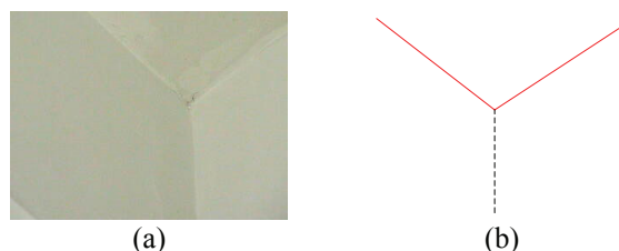
Fig. 2 Illustration of house corner. (a) A real house corner. (b) The two edge lines of a house corner used for vehicle location in this study (vertical dotted line is not used).
