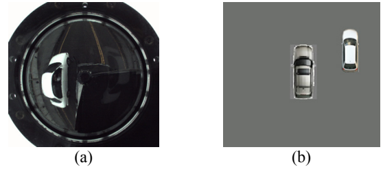
Fig. 14: Detecting static nearby car from moving vehicle. (a) Original image. (b) Generated surround map (direction of car is 180^\circ reversed when compared with real situation in (a)).
