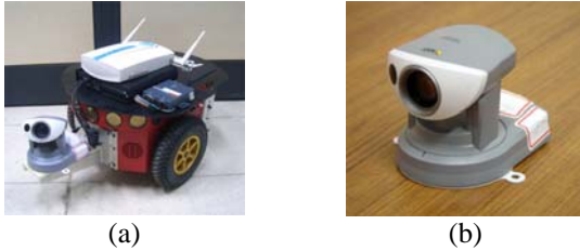
Fig. 1 The test bed used in this study. (a) The vehicle. (b) The PTZ camera.
