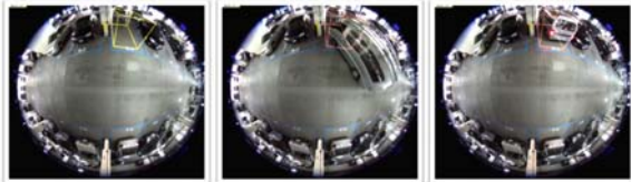
Fig. 12: An example of empty parking-space detection.
