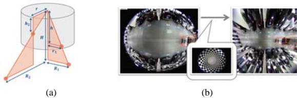
Fig. 5: Mapping from fisheye images to top-view images. (a) An illustration of notations involved in the mapping. (b) An experimental result.
