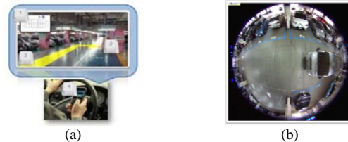
Fig. 1: Proposed AR-based guidance system for car parking. (a) An illustration. (b) An image of a parking lot used in proposed system.
