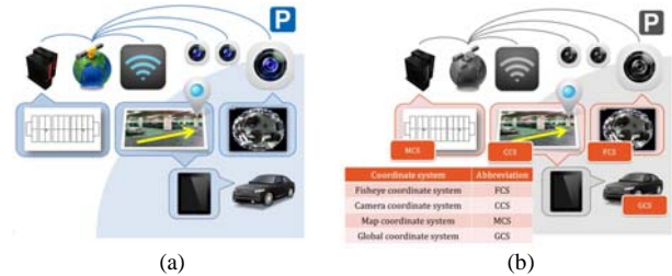
Fig. 2: Hardware architecture of proposed system.
