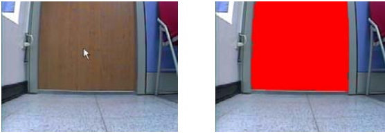
Fig. 9 A learning process of choosing a door manually. (a) Choosing a door. (b) A door region is obtained.
