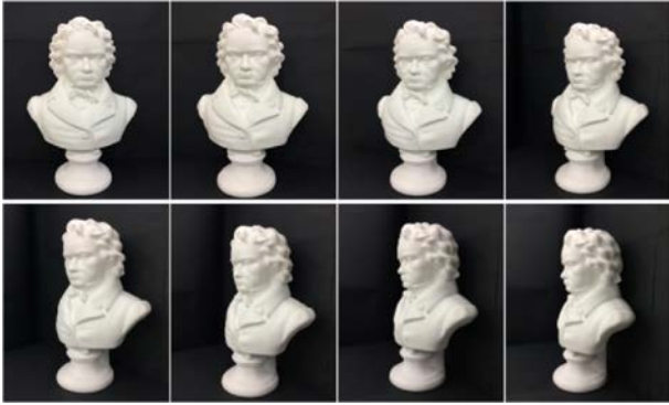
Fig 3. Images taken of a single statue from different view angles with 10 degrees interval in a 180° range.
