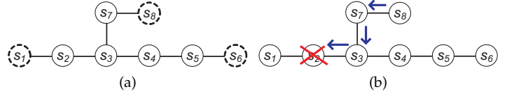
Fig. 17: Deal with network partition by mobile sensors: (a) initial network topology, where dominated nodes are marked by dashed circles and (b) cascaded movement when s_2 fails.
