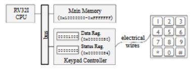
Its LSB bit is the REDAY bit that indicates whether the keypad was pressed since the last time the CPU read a value from the data register
