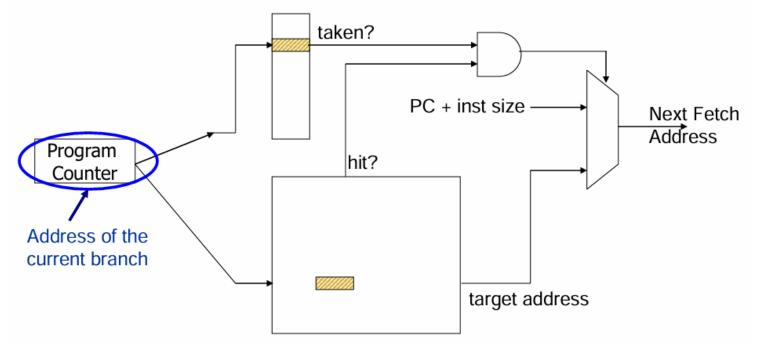
Cache of Target Addresses (BTB: Branch Target Buffer)
