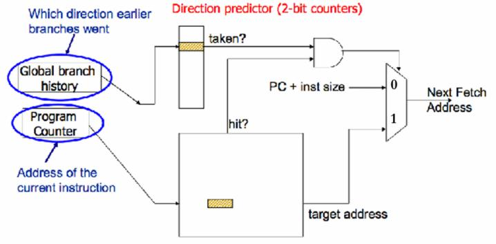
Cache of Target Addresses (BTB: Branch Target Buffer)
