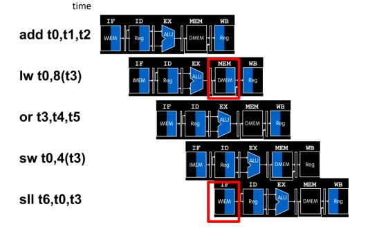
RV32I separates IMEM and DMEM to avoid structural hazard
