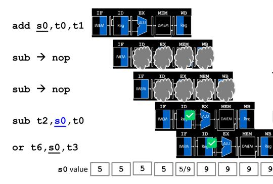
Stalls reduce performance 1. Compiler could rearrange code/insert nops to avoid hazard (and therefore stalls), but this requires knowledge of the pipeline structure
