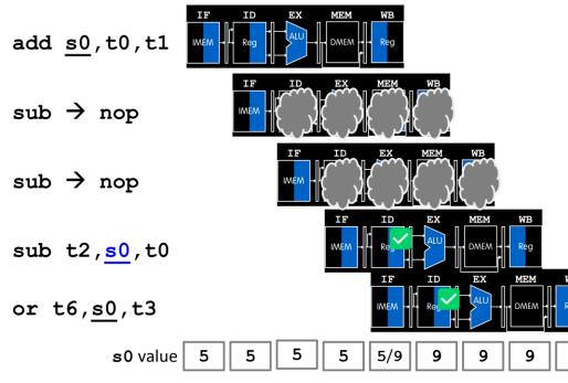
"Bubble" to effectively nop: 1. Affected pipeline stages do nothing during clock cycles 2. Stall all stages by preventing PC, IF/ID pipeline register from
