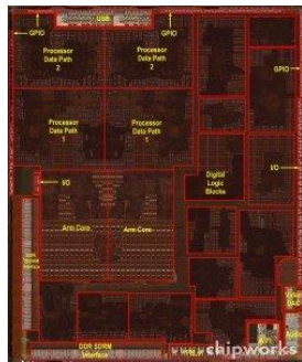
2010 Apple A4 65 nm TSMC 53 mm 2 4 accelerators
