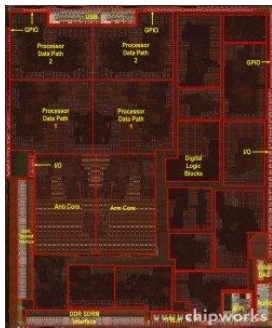
2010 Apple A4 65 nm TSMC 53 mm 2 4 accelerators
