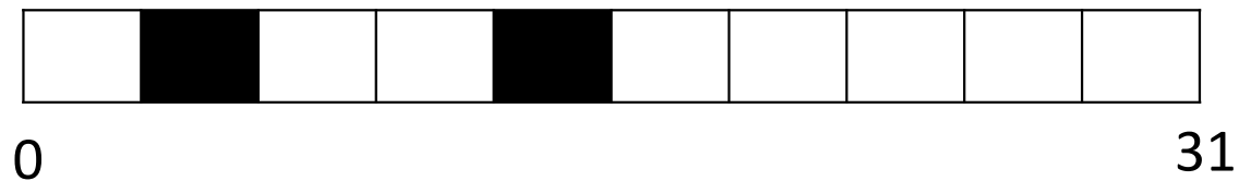
Memory layout of the buddy allocator
