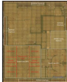
2014 Apple A8 20 nm TSMC 89 mm 2 28 accelerators
