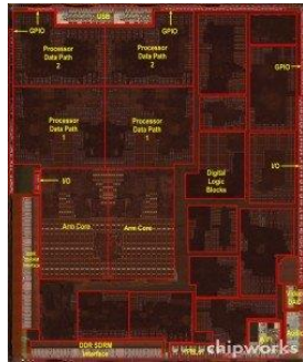
2010 Apple A4 65 nm TSMC 53 mm 2 4 accelerators
