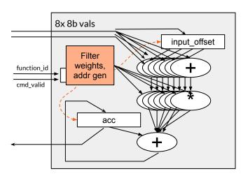
Move re-used data (filter weights) into the CFU
