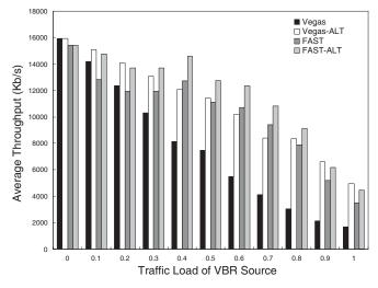
Fig. 4. Four TCPs' average throughput vs. different backward traffic loads.
