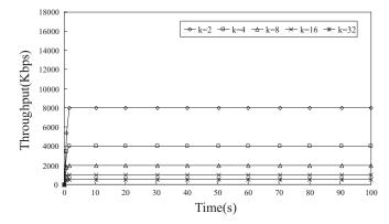
Fig. 2. Throughput of Vegas in asymmetric networks.
