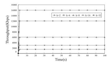
Fig. 3. Throughput of Vegas-ALT in asymmetric networks.
