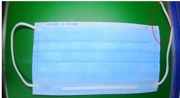
Figure 4: Mask with Ear Strap Breakage.
