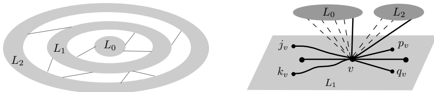
Figure 6.1: (a) A 3-outerplanar graph with levels \mathbf{L}_0 , \mathbf{L}_1 , and \mathbf{L}_2 . (b) Local connections w.r.t. a vertex v . Bold edges represent edges to be kept in the edge reduction process, while dashed edges represent edges to be removed.
